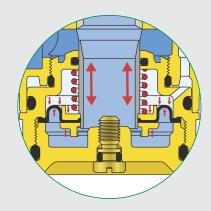
Valve **B** regulates flow rate G by changing the flow path cross section.
