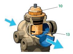
Turning adjustment nut (10), which determines the number associated with the "Adjustment position", results in opening/closing of the bore cross section in the external obturator (13). Hence, each bore cross section set on the adjustment nut corresponds to a specific Gmax value.
